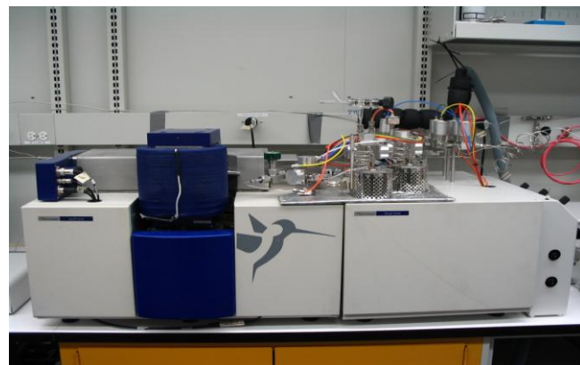
Figure 2 : Picture of a gas source isotope ratio mass spectrometer.
